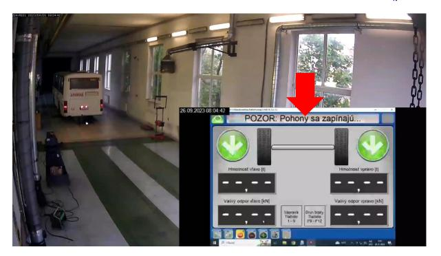
Vehicle (bus) of the **driving school** (major defect on rear brakes - brake force imbalance over 30%)
